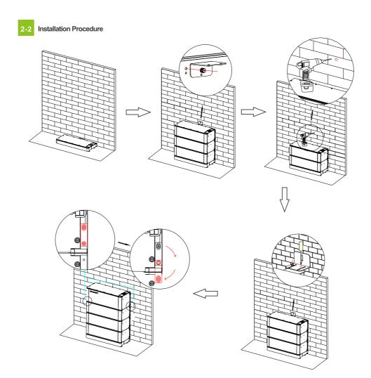
Note: The safety part needs to be installed at the top battery, however, once the number of the battery pack is higher than 7, one more safety part should be installed in the middle battery which is shown the last step.
